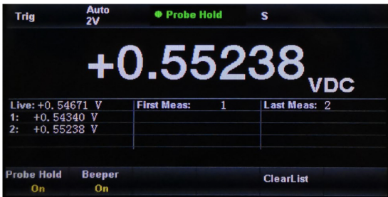
199999 count, 4.3 inch TFT LCD display, Hold measurement function
