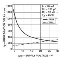
Figure 12. Propagation delay vs. supply voltage.
