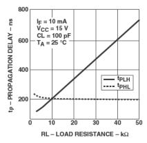
Figure 10. Propagation delay vs. load resistance.
