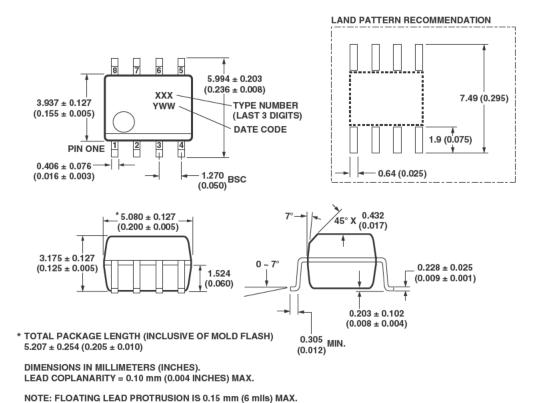
NOTE: FLOATING LEAD PROTROSION IS 0.15 IIIIII (6 IIIIIS) MAX
