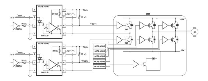
Figure 24. Typical application circuit.
