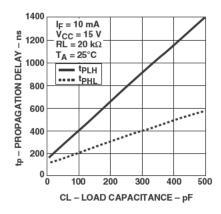
Figure 11. Propagation delay vs. load capacitance.
