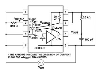
Figure 19. AC equivalent circuit for Figure 18 during common mode transients.
