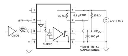
Figure 15. Recommended LED drive circuit.
