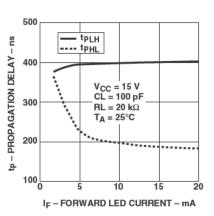
Figure 13. Propagation delay vs. input current.
