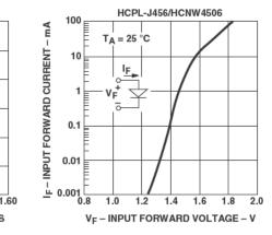
Figure 4. HCPL-4506 and HCPL-0466 input current vs. forward voltage.
