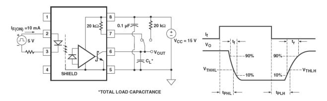
Figure 6. Propagation delay test circuit.
