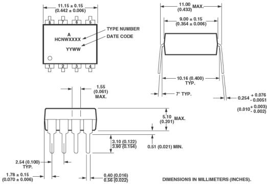
NOTE: FLOATING LEAD PROTRUSION IS 0.25 mm (10 mils) MAX.
