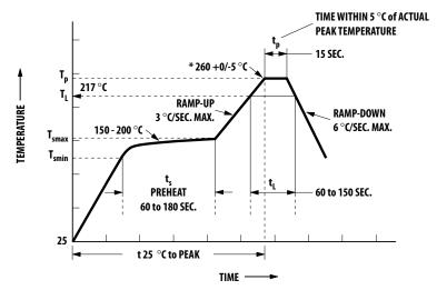
NOTES: THE TIME FROM 25 °C to PEAK TEMPERATURE = 8 MINUTES MAX.  $T_{smax}$  = 200 °C,  $T_{smin}$  = 150 °C
