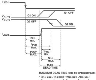
= (t<sub>PLH</sub> MAX. - t<sub>PHL</sub> MIN.) - (t<sub>PLH</sub> MIN. - t<sub>PHL</sub> MAX.) = PDD\* MAX. - PDD\* MIN.
