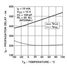
Figure 9. Propagation delay with internal 20  $k\Omega$  RL vs. temperature.
