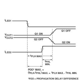
NOTE: THE PROPAGATION DELAYS USED TO CALCULATE PDD ARE TAKEN AT EQUAL TEMPERATURES.
