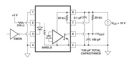
Figure 18. LED drive circuit with resistor connected to LED anode (not recommended).
