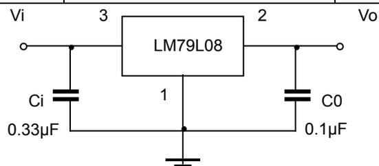
Note: Bypass capacitors are recommended for optimum stability and transient response and should be located as close as possible to the regulators.
